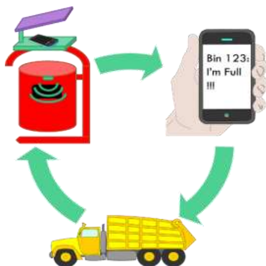
Fig 5.7: Basic operation of the system
